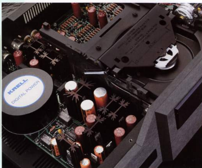
CD-1 internal layout, left to right: power supply, transport and analog outputs, digital processing.
