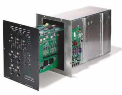
A fully programmable digitally-controlled active crossover ensures seamless integration between the Master Reference Subwoofer and the main loudspeakers. Powerful Krell software controls the simultaneous connection of conventional and LFE inputs for maximum subwoofer performance in music and home theater systems. Up to five user-definable settings for filter parameters—such as slope, type, and frequency—can be
