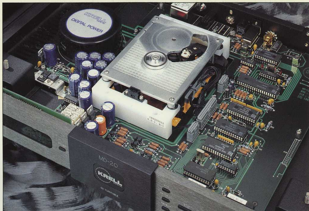
An interior view of the MD-20 reveals its robust and clean construction. Leveling feet, which provide superb vibration isolation, are enclosed in housings at the corners of the chassis. Power supplies are in close proximity to the transformer, at left. Control circuitry for transport, display and programming operations is to the right of the transport subassembly.
